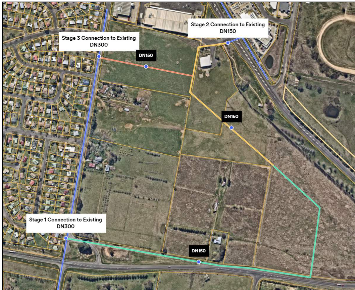
Figure 3.3.1 – Connections to Council's Water Supply Network
